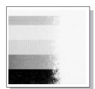
The second sample, left, shows an incorrectly set "media width adjustment". For 4-inch or 100mm wide media, the adjuster should be set to the "9" position on the blue dial.
