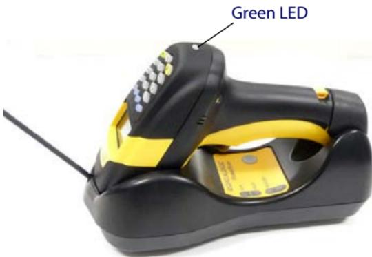
If it ever becomes necessary to change the reader, just read the bind-address label applied to the cradle and position the new reader onto the cradle.
